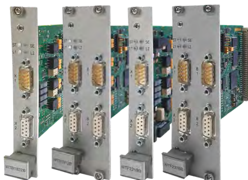
EKE-Trainnet® Wire Train Bus Interface Module
