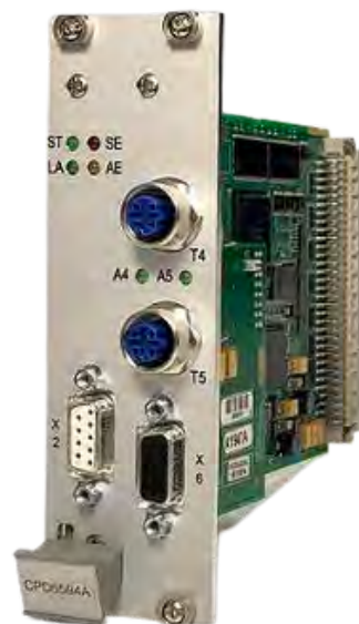
EKE-Trainnet® Central Processing Unit with Dual Homing
