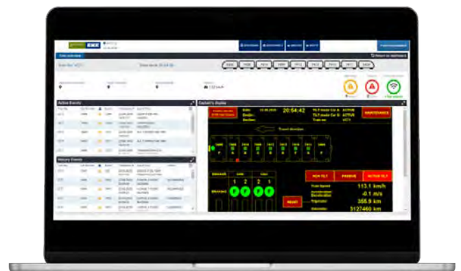
Example of SmartVision™ Remote Diagnostics with driver's display
