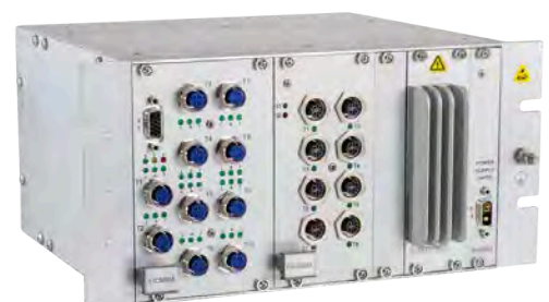
TCN Gateway with Ethernet Switches
