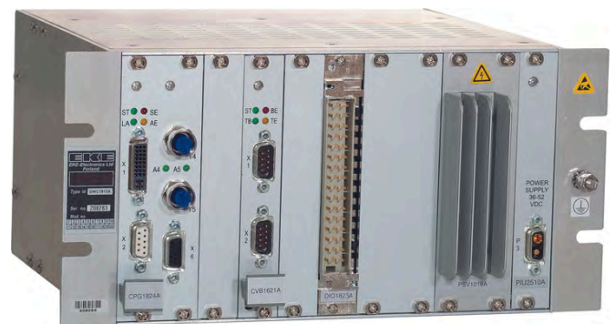
Vehicle Control Unit with CAN and Digital Input/Output Interfaces
