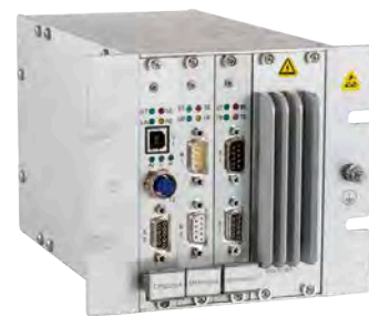
TCN Gateway with CAN Interfaces
