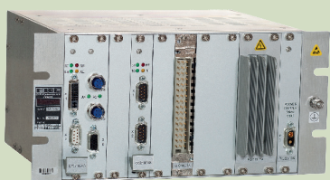
VCU with CAN and Digital Input/Output Interfaces
