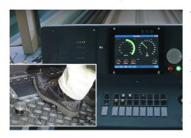
The EKE-Trainnet® Vigilance Control System (VCS) known also as Dead Man's Switch or Driver Safety Device (DSD) monitors the train driver's vigilance at all times. The system automatically stops the train if the driver is unable to periodically press the pedal or button of the system. The Trainnet® VCS can be customized for different alarm periods or modified system setups.
