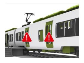
The EKE-Trainnet® Automatic Selective Door Operation (ASDO) is developed to improve passenger operation at stations where the platforms are shorter than the trains. ASDO enables an automatic check of the train's position and the platform configuration so only the doors that can be safely opened are released. Passenger comfort and safety is enhanced while allowing for shorter stops at stations.
