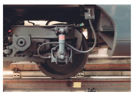
The EKE-Trainnet® Hot Axle Box Detection (HABD) is an on-board monitoring system that observes hot axle box bearing and gearbox temperatures. The system improves train safety by detecting wheelset bearings and gearbox presenting a risk of failure. The temperature sensors monitor the hot axle box grease temperature at all times, and the train computer issues warnings if the measurements vary from the normal. The EKE-Trainnet® HABD follows the EN 15437-2 standard.
